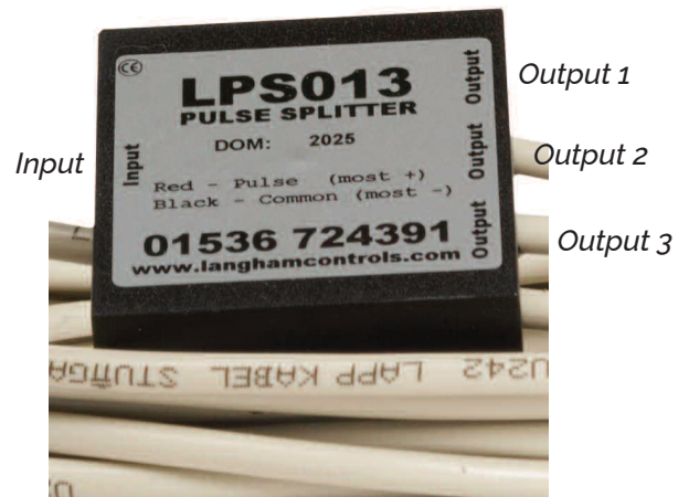
3 way Pulse Splitter – LPS013
